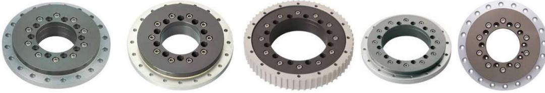
iglidur® PRT is a slewing ring bearing with the proven advantages of the igus® polymer bearings. The sliding elements made of iglidur® J operate absolutely maintenance and lubrication free. The mating rings of the slewing bearing are made of aluminium or stainless steel; the mating surfaces of iglidur® J sliding elements are hard-anodised. All fastening screws are made of stainless steel.
