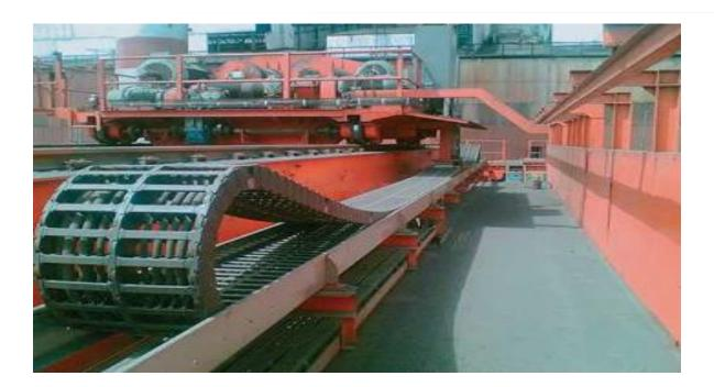
Reliable and dynamic cable management is one of the greatest challenges in modern crane technology. Virtually all modes of crane applications are facing intensifying requirements regarding travel distances, speeds and precision.
